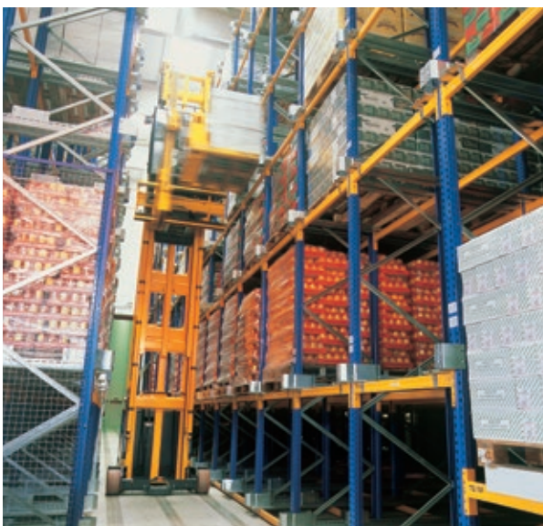
Hochregallager high rack storage area
